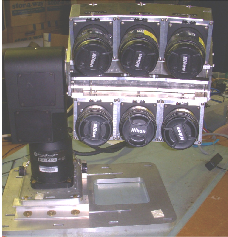
Figure 16: Finished Camera Head Front View
